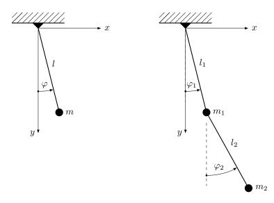
We neglect the masses of the rods l,  $l_1$ ,  $l_2$  and consider the masses m,  $m_1$ ,  $m_2$  as point masses. I.e. we consider the pendulums as mathematical pendulums.
